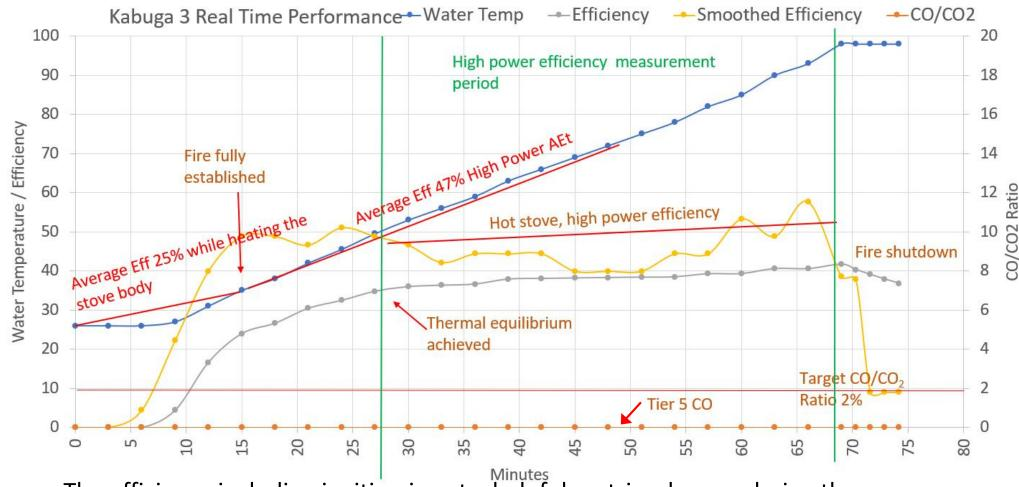
The efficiency including ignition is not a helpful metric when analysing the performance of a high mass institutional stove. We determined the thermal efficiency after the system reached thermal equilibrium ( $AE_T$ )which typically takes 25 to 45 minutes. After this point, the heat gain rate of the pot is constant. If the firepower is changed, wait until  $AE_T$  is achieved before making a determination. Above, the  $CO/CO_2$  ratio is so low it does not show above the axis. PM is negligible.
